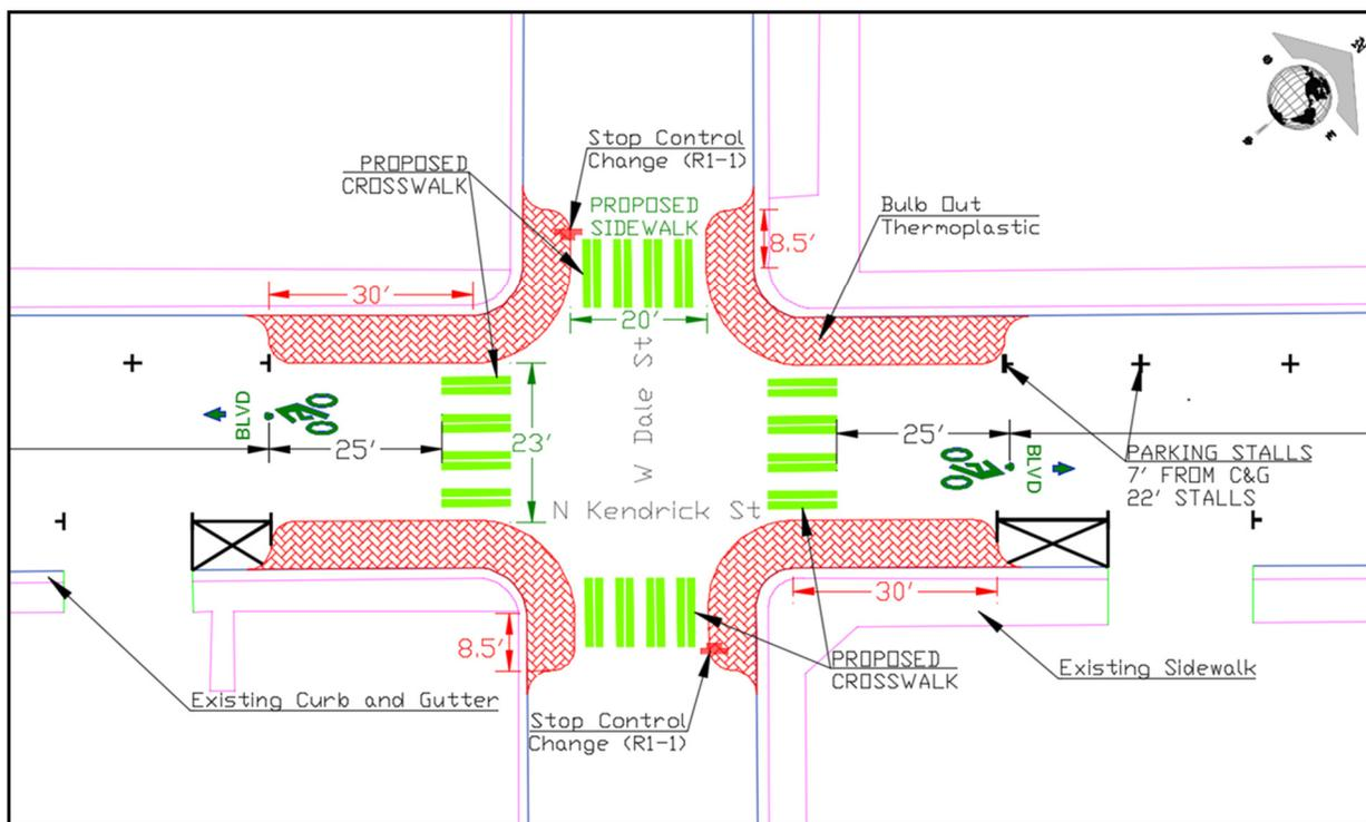
Figure 19: Bulb-Out Traffic Calming Treatment at Kendrick Street and Dale Avenue
