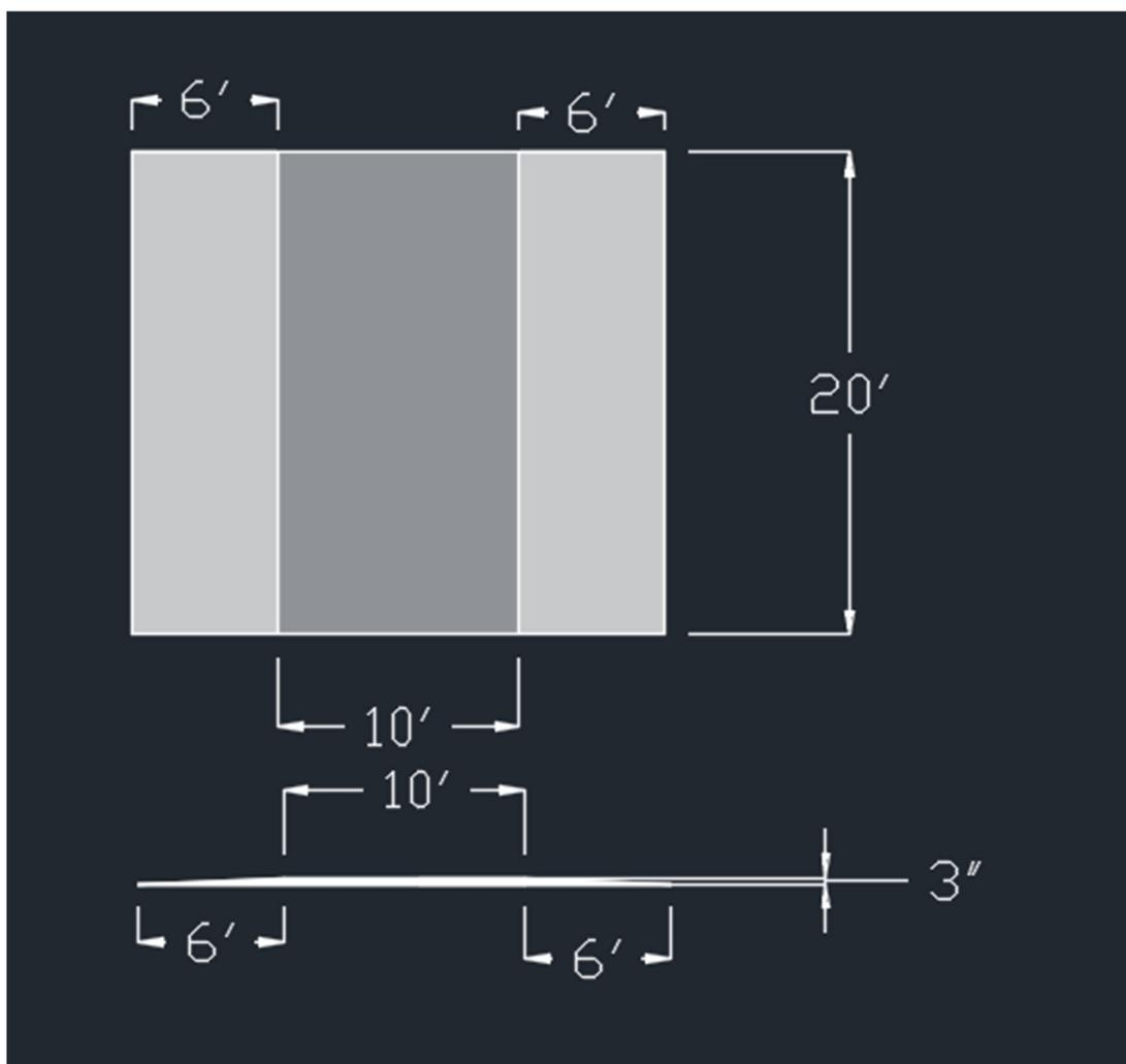
Figure 20: Speed Table Detail
