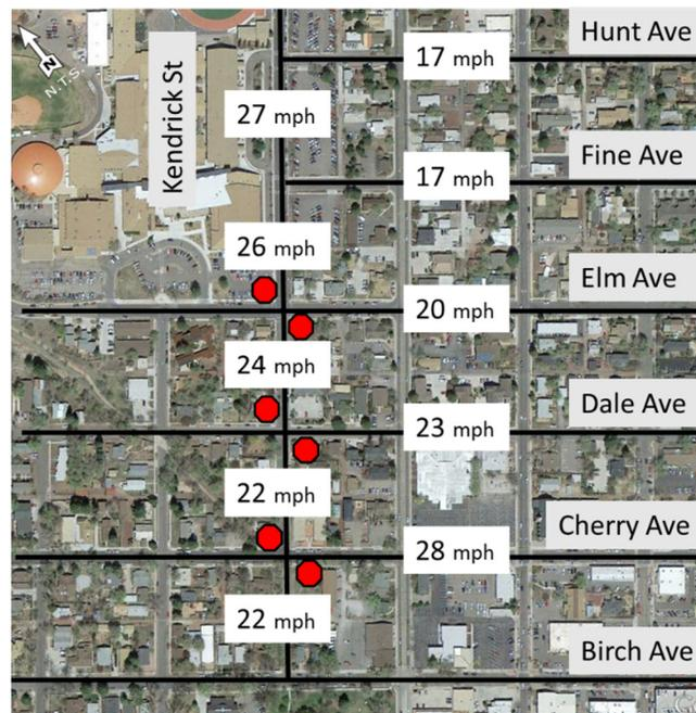
Figure 10: 85<sup>th</sup> Percentile Speeds for Vehicles in Project Area [3]
